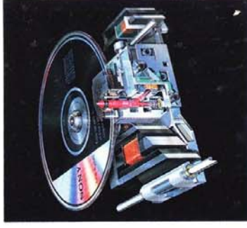
Sony's Linear Motor Tracking Mechanism assures extremely quick location of CD selections.
